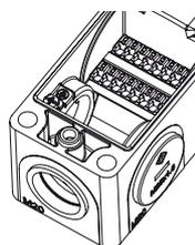
The switch is provided with a PUSH-IN type spring connection system on the inside. This technology allows a very handy quick wiring procedure, since the wire just needs to be inserted into the appropriate hole in order to be secured and to establish the electrical connection. The said operation can be carried out without the help of any tool, but simply using rigid or flexible wires with wire-end sleeves. Release is obtained by pressing the appropriate wire-releasing button.
