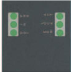
As the LEDs have been designed for quick immediate diagnosis, the status of each input and output is highlighted by one specific LED. This makes it possible to quickly identify the interruption points in the safe chain, which device is released, which door is opened and any errors inside the device. All that in a straightforward way without needing to decode complex blinking sequences.
